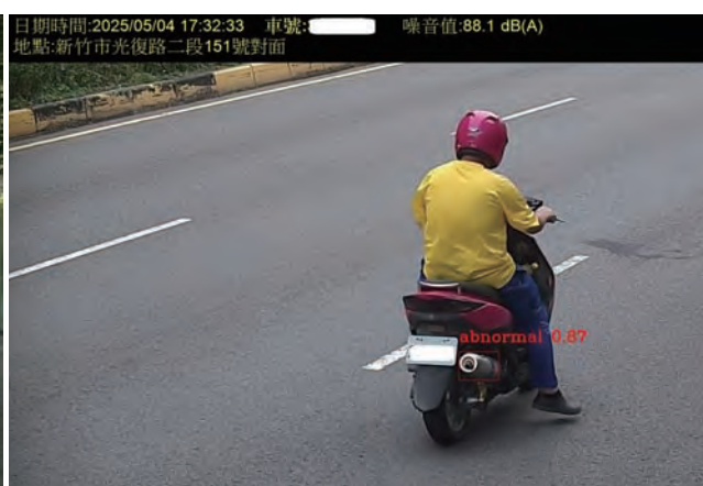
Vehicular Six-in-One System into vans / AI Automatic Judgment and Inspection of Modified Exhaust Pipes of Motorcycles
