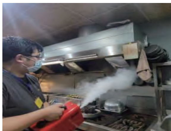
Covering of Dustproof Nets in Exposed Construction Areas to Inhibit Dust / Use of Technological Instruments to Visualize the Smoke Flow and Confirm the Collection Effect of the Hood
